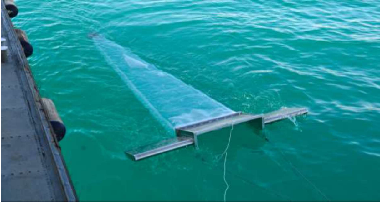
Figure 6-2. All tows should be conducted from the ship's side and beyond the ships' wake (Photo © Th. Vlachogianni).
