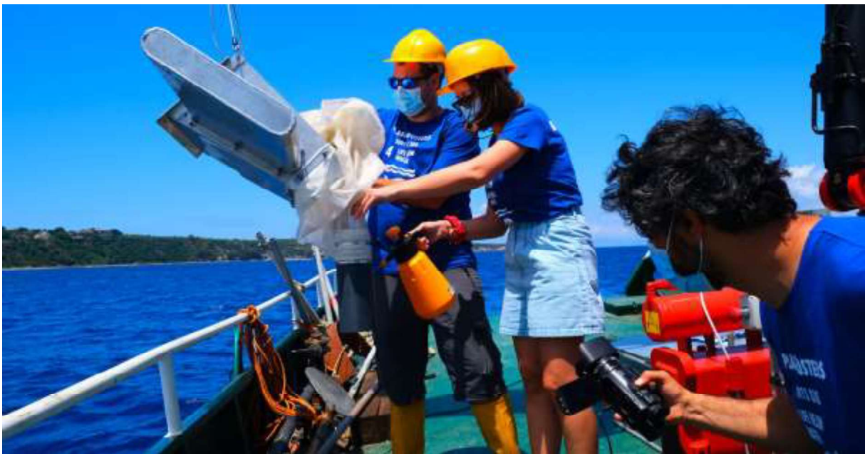
Figure 6-3. After completion of each tow, the net should be washed thoroughly from the outside with filtered seawater (Photo © Th. Vlachogianni).
