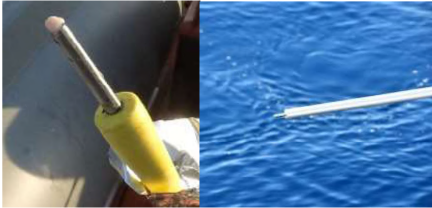
Figure 15-6. Arrow and tip (left) and tip on the aluminum pole (right) with the collected biopsy.
